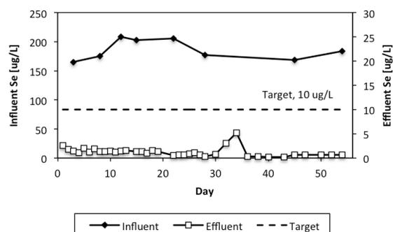
**Figure 1.** EBR bench scale total selenium removal from Water A. Effluent target concentration presented for comparison.
