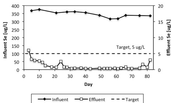
**Figure 4.** EBR bench scale total selenium removal from Water D. Effluent target concentration presented for comparison.
