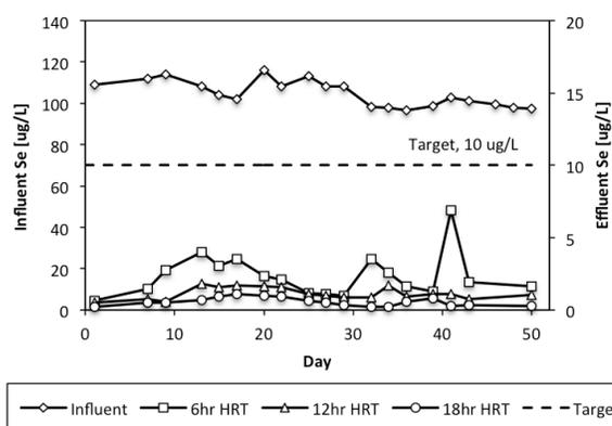
**Figure 6.** EBR pilot scale total selenium removal throughout the system at 6, 12, and 18 hour hydraulic retention time (HRT).
