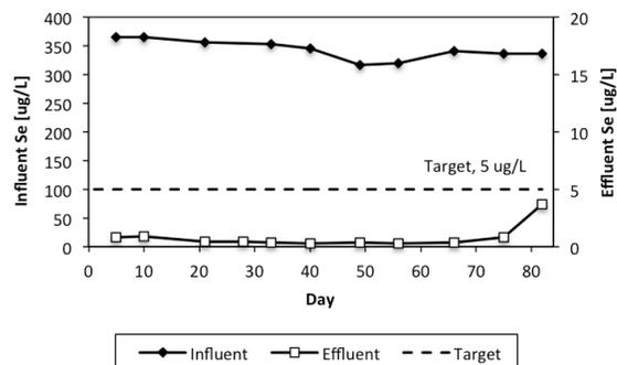
**Figure 5.** EBR bench scale dissolved selenium removal from Water D. Effluent target concentration presented for comparison.
