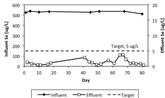
**Figure 3.** EBR bench scale total selenium removal from Water C. Effluent target concentration presented for comparison.
