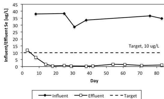
**Figure 2.** EBR bench scale total selenium removal from Water B. Effluent target concentration presented for comparison.
